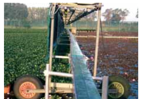
Before the winter the plants are brought inside using the conveyor belt.
